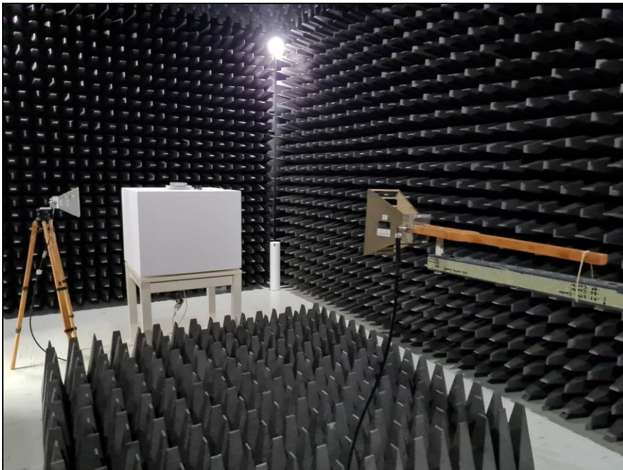
Figure 11: Radiated Emissions (1 – 6GHz)
