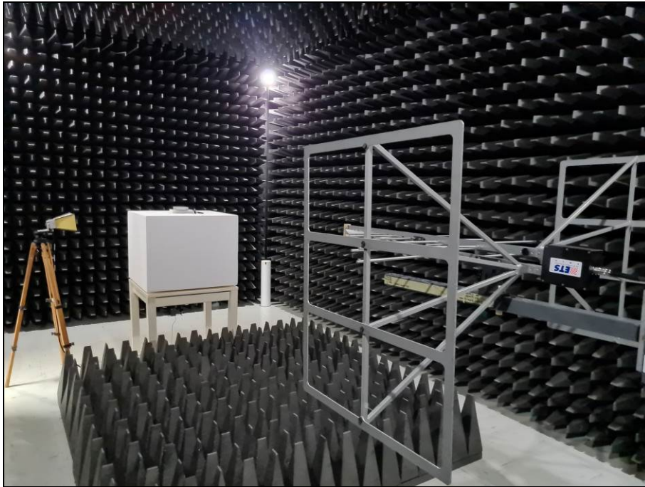
Figure 10: Radiated Emissions (30 – 1000MHz)
