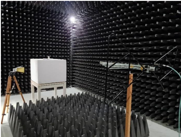
Figures 11 & 12: Measurement Setup for Radiated Emissions between 30 MHz and 4 GHz
