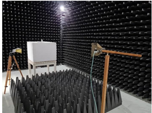
Figures 11 & 12: Measurement Setup for Radiated Emissions between 30 MHz and 4 GHz
